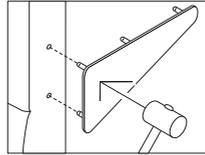
Place the bracket against the mounting holes of the element on the right and tap it in with a rubber hammer until it is flush with the element.
