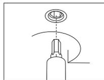
Tighten the set screws (located on the bottom of the shelf) using a 4 mm Allen key.
