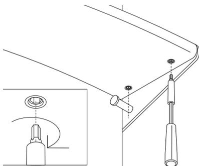
Tighten the set screws (located on the bottom of the shelf) using a 4 mm Allen key
