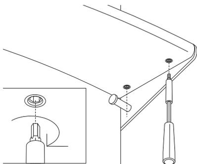
Tighten the set screws using a 4 mm Allen key.
