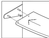
Push the shelf onto the bolts of the bracket.
