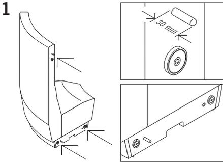
Affair elements are always connected without tools. Two elements are positioned one below the other by means of a bolt and held together by magnets.
