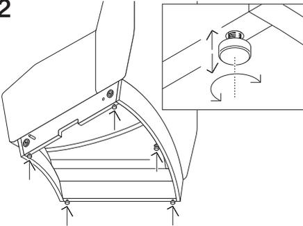
All Affair elements are equipped with levelling glides. These glides can be unscrewed approx. 20 mm.
