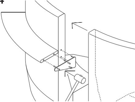
Place the bracket against the mounting holes of the element in the middle and the shelf and tap it in with a rubber hammer until it is flush with the element.
