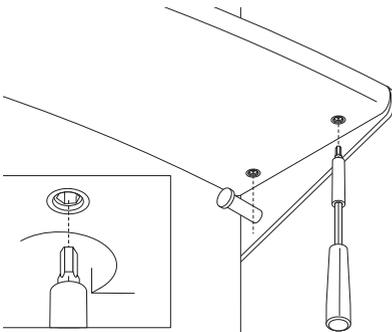
Tighten the set screws (located on the bottom of the shelf) using a 4 mm Allen key.
