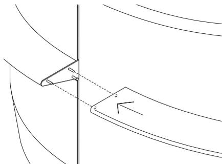
Push the second shelf onto the bolts of the bracket.
