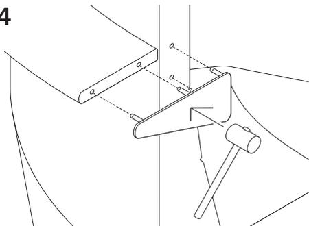
Place the bracket against the mounting holes of the element on the left and the shelf and tap it in with a rubber hammer until it is flush with the element.
