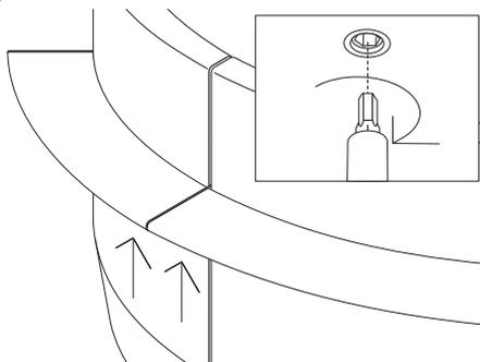
Tighten the set screws (located on the bottom of the shelf) using a 4 mm Allen key.
